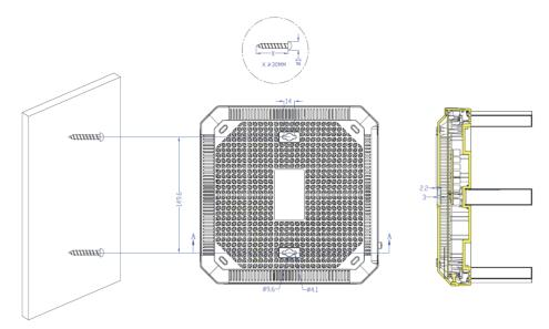
Note: The diameter of the screw, 3.5mm<D<6mm, and the distance of two screws is 149.6mm. The screw that project from the wall need around 4mm based, and the length of the screw need to be at least 30mm to withstand the weight of the product.
